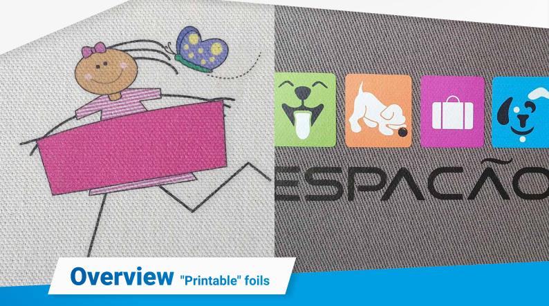
So-called "printable" foils are printable flex foils that are processed with a print & cut device. Depending on the version, these foils can be printed with eco-solvent, solvent, latex inks and UV inks and are contour-cut immediately after printing. A transfer tape is needed for the transfer to textiles.
